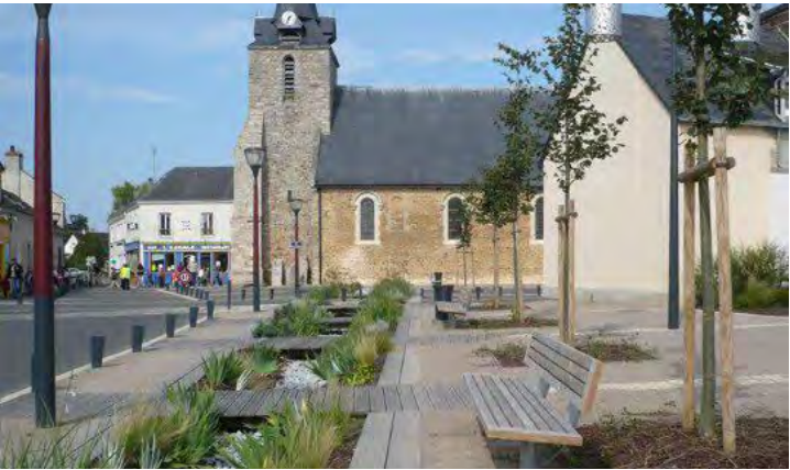
Swales capture runoff from surrounding areas.
