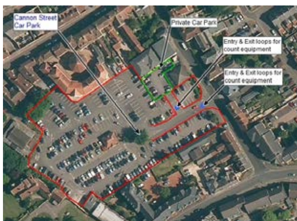
Figure 2, Canon Street Car Park overview with location of count loops
