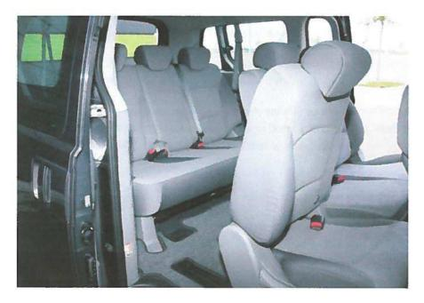
The second image shows the middle row seating with the quick-release lever which operates the drop forward middle seat. The near-side seat is similar.
