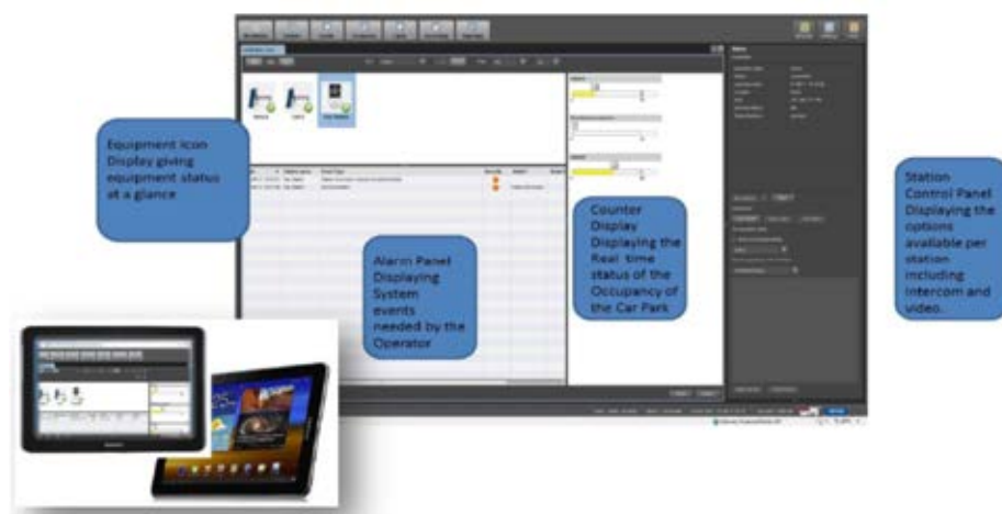
Figure 15, PoF central system user interface
